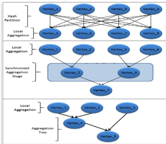
Fig. 2: Three Distributed Grouped Aggregation Approaches: Hash Partition, Hierarchical Aggregation, and Aggregation Tree.
