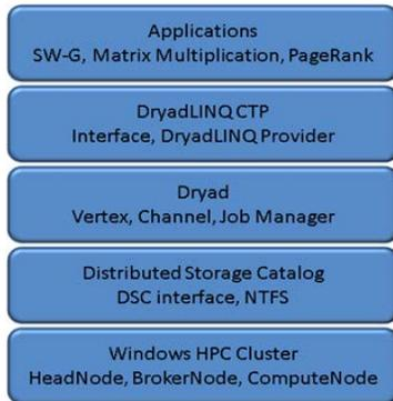
Fig. 1: Software Stack for DryadLINQ CTP
